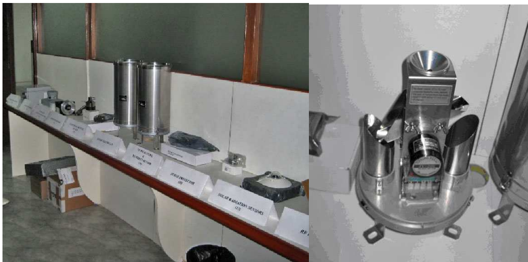
Figure 2.11: Equipment on Display for Inspection and Tipping Bucket Raingauge
